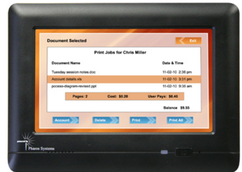
The Omega PS200 displays all of the user's queued print jobs, the cost of each job, and the total cost of all jobs selected.
